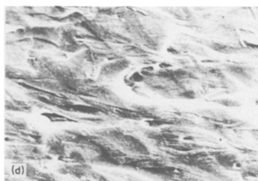
Figure 5 SEM micrographs of the fracture surface of a dry methanol craze in polystyrene; crack propagation is from (a) to (d).
